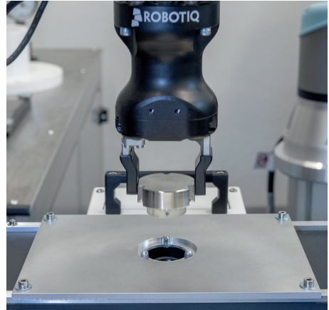
Figure 3: Robotic gripper with specimen holder above x-y microscope stage.
