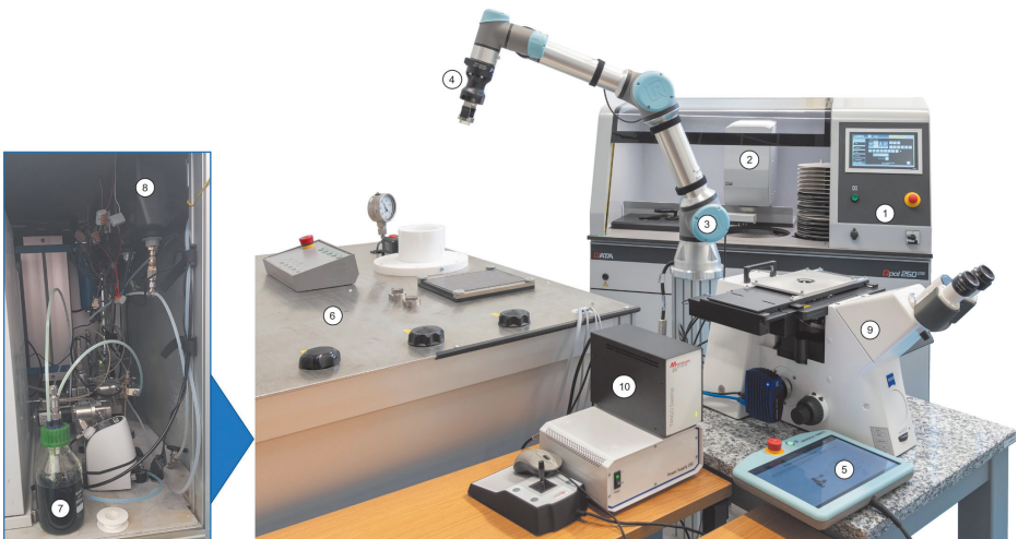
Figure 1: The RASI system and its main components: 1 – QATM, QPOL 250 Bot, 2 – preparation robot, 3 – Universal Robots, UR5e, 4 – robotic gripper, 5 – robot terminal, 6 – etching unit, 7 – acid container, 8 – water and ethanol containers, 9 – Zeiss, Axio Observer 7, 10 – microscope power supply.
